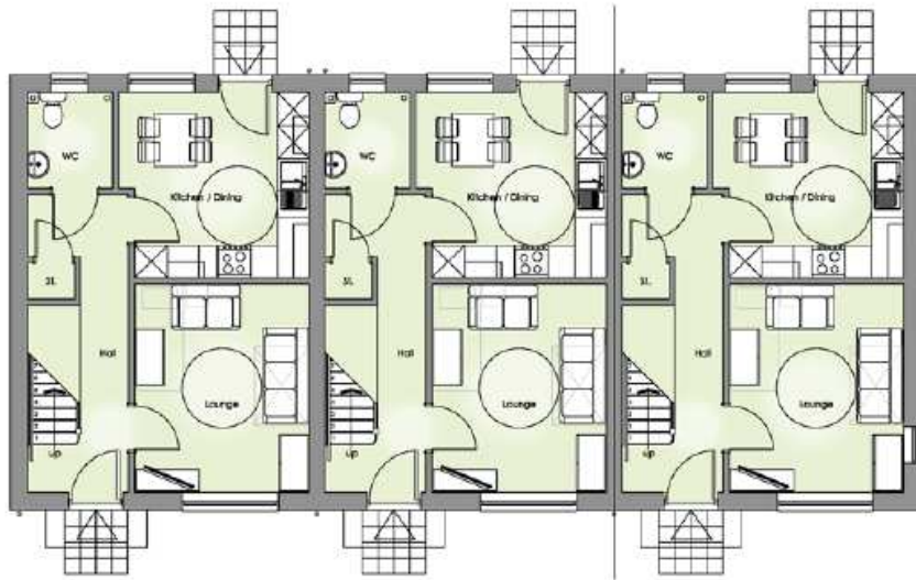
Ground Floor Plan Type 2B (4.2.1)
